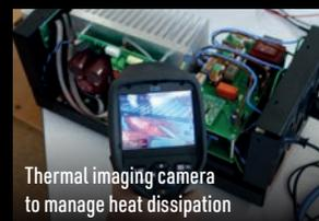
Thermal imaging camera to manage heat dissipation
